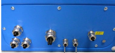
Threaded fittings M12 for relay outputs
