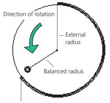
Tape measure length on the outer surface of the rotor
