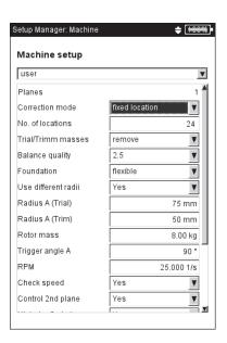
\*This parameter can be changed in each balancing run (MENU - Tools)
