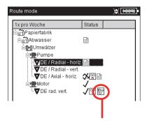
Measurement location contains 'Multimode' measurement results
