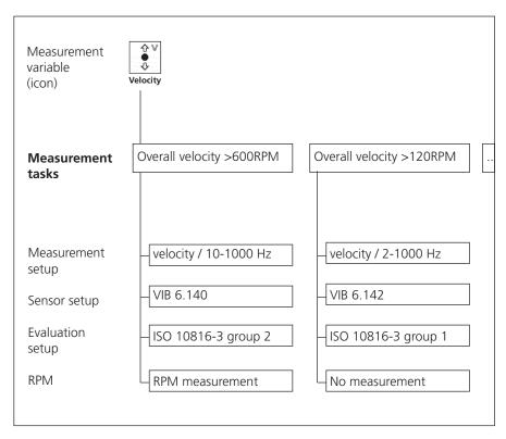
The measurement tasks are sorted according to measurement variable\* and assigned a measurement icon in the selection screen. If you are in the 'Multimode' operating mode for example, all measurement tasks of the 'Vibration velocity - Characteristic value' measurement variable appear under the icon shown above. The letters 'a', 'v', and 'd' in the icon stand for 'Acceleration', 'Velocity' and 'Displacement'.
