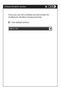
When a default sensor has been set up, the sensor can no longer be specified in the measurement task manager. The corresponding field is grayed out, although the sensor originally specified is still visible.
