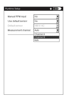
Use this option when you do not have an RPM sensor on the route and need to perform measurements that require the RPM (e.g. roller bearing condition, order-based spectra). If the measurement task already has information on the RPM, this option is ignored.
