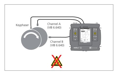
The signals of both sensors are displayed either as individual signals or as an orbit in a polar chart. The maximum and minimum phase vectors and the order filter are displayed in the data field on the orbit display. The angular coordinate of the cursor indicates the angular distance to Keyphaser point\*, which is marked in the orbit with an arrow. To check the phase stability, multiple rotations of the shaft can be displayed in the orbit diagram.
