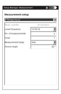
Sensor angle (Orbit): The angle between the two sensors can be freely selected between 5° and 175°.
