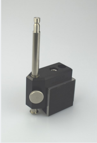
Plunger mounted on magnetic foot
