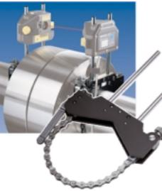
Quite possibly the only bracket you'll ever need: the standard ROTALIGN® PRO compact chaintype bracket ALI 2.891set uses interchangeable parts to fit onto shafts and solid couplings ranging from 15 mm to 500 mm (5/8" to 20") in diameter in a matter of seconds!
