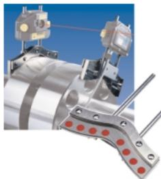
Shafts can't be rotated? No problem with ROTALIGN® PRO! Simply place the ALI 2.230 magnetic sliding bracket onto the coupling flange or shaft end and slide it around the circumference to take measurements in seconds. Suitable for shaft/coupling diameters from approx. 80 mm (3 1/8") on up.
