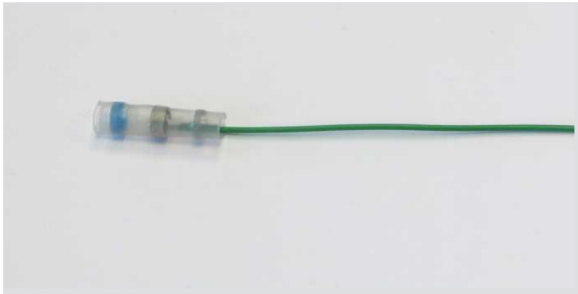
Solder sleeve with ground lead (green)
