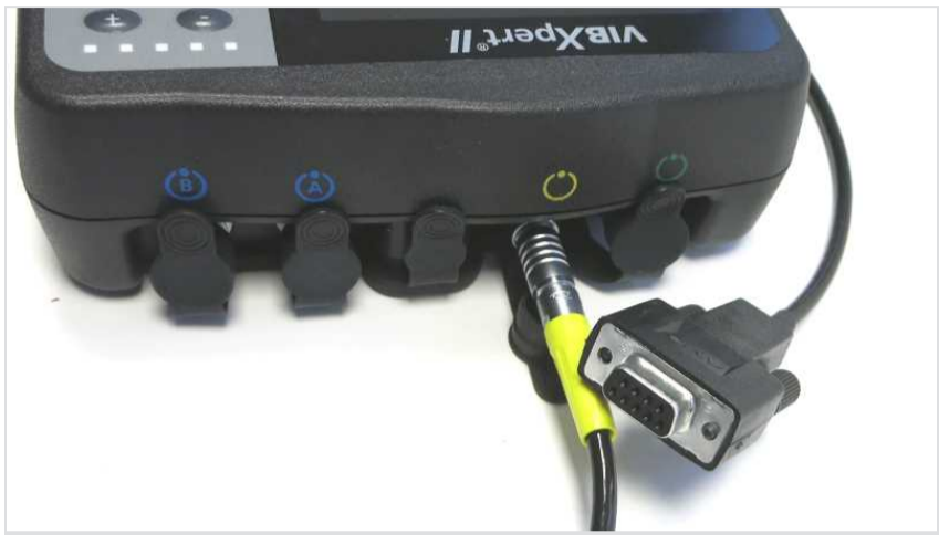
Serial PC cable connected to VIBXPERT II
