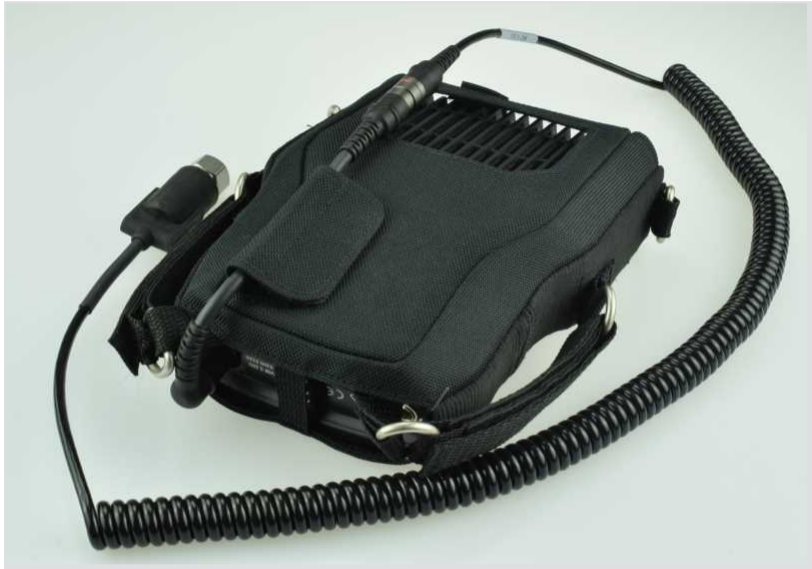
Accelerometer VIB 6.142R connected to VIBSCANNER 2 with sensor cable VIB 5.236 and safety release cable VIB 5.239.
