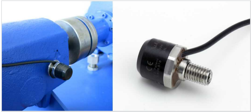
Mini accelerometer can be installed on limited space
