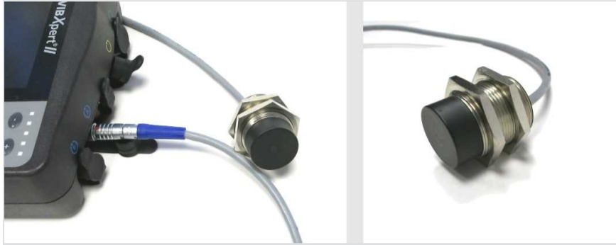
Displacement sensor connected to VIBXPART II
