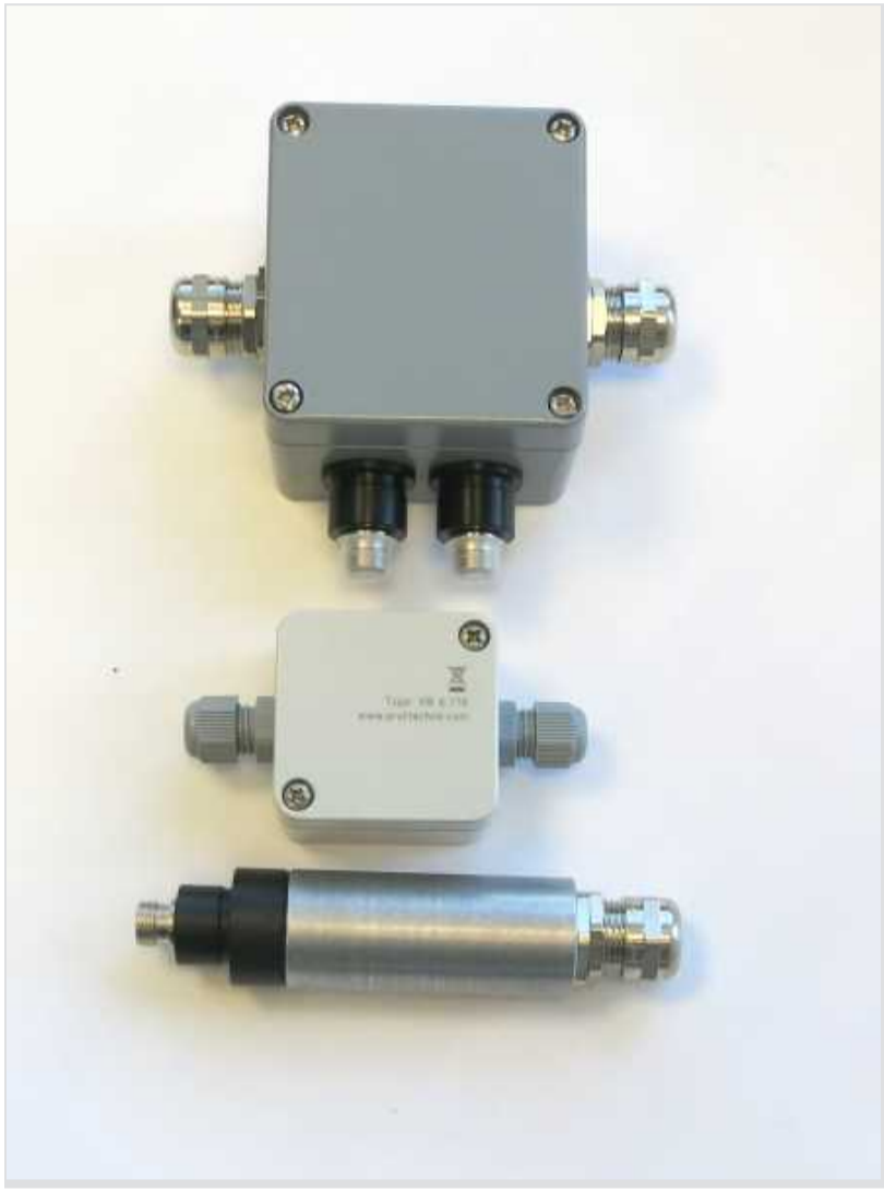
Junction boxes used for the extension of two cables (top) and for one cable (middle and bottom)
