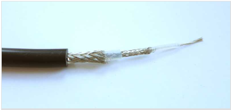
Triaxial cable with double shielding.
