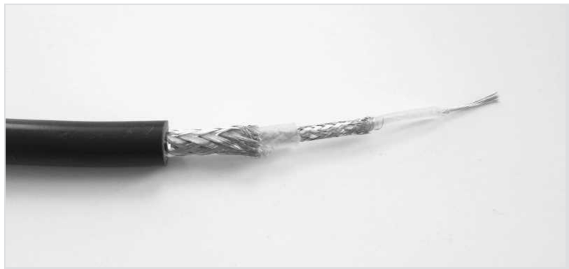
Triaxial cable with double shielding.
