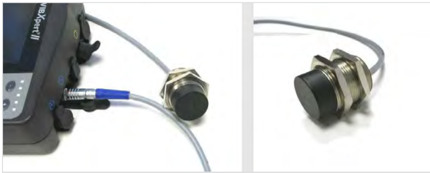
Displacement sensor connected to VIBXPERT II
