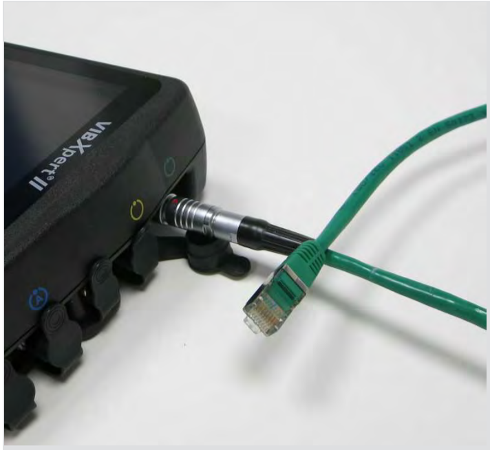
Ethernet cable connected to VIBXPART II
