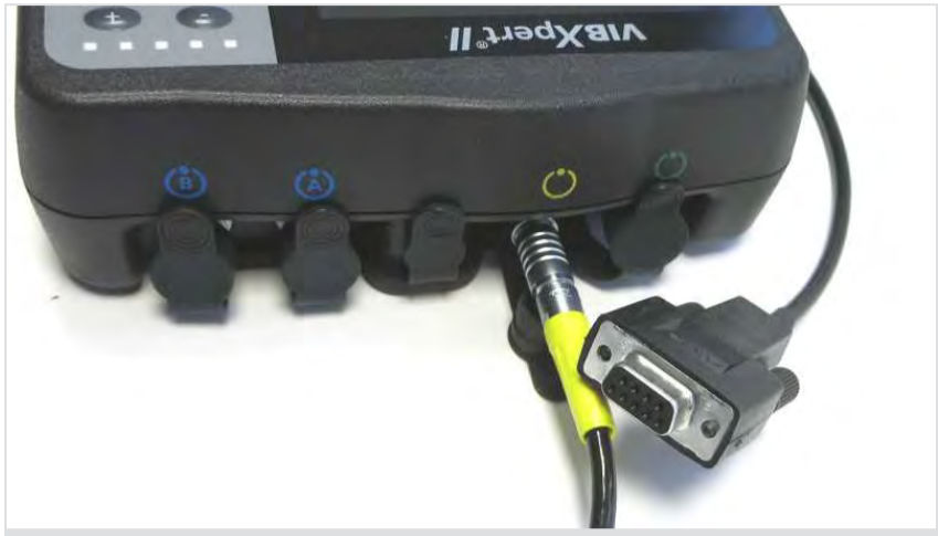
Serial PC cable connected to VIBXPERT II
